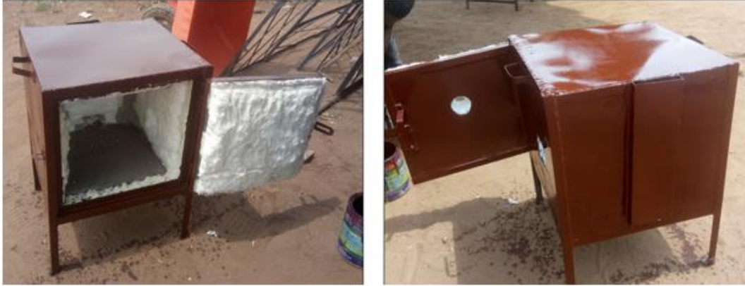
Figure 4. Photograph of the constructed test kiln.
