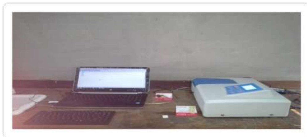
Plate 1: A digital UV visible MetaspecAE1405031Pro spectrophotometer interfaced with a dedicated PC that uses the spread sheet of a Metaspec pro-[multi-wavelength analysis (mw11611300004)] software. (Mbabuiket. al. , 2018*).
